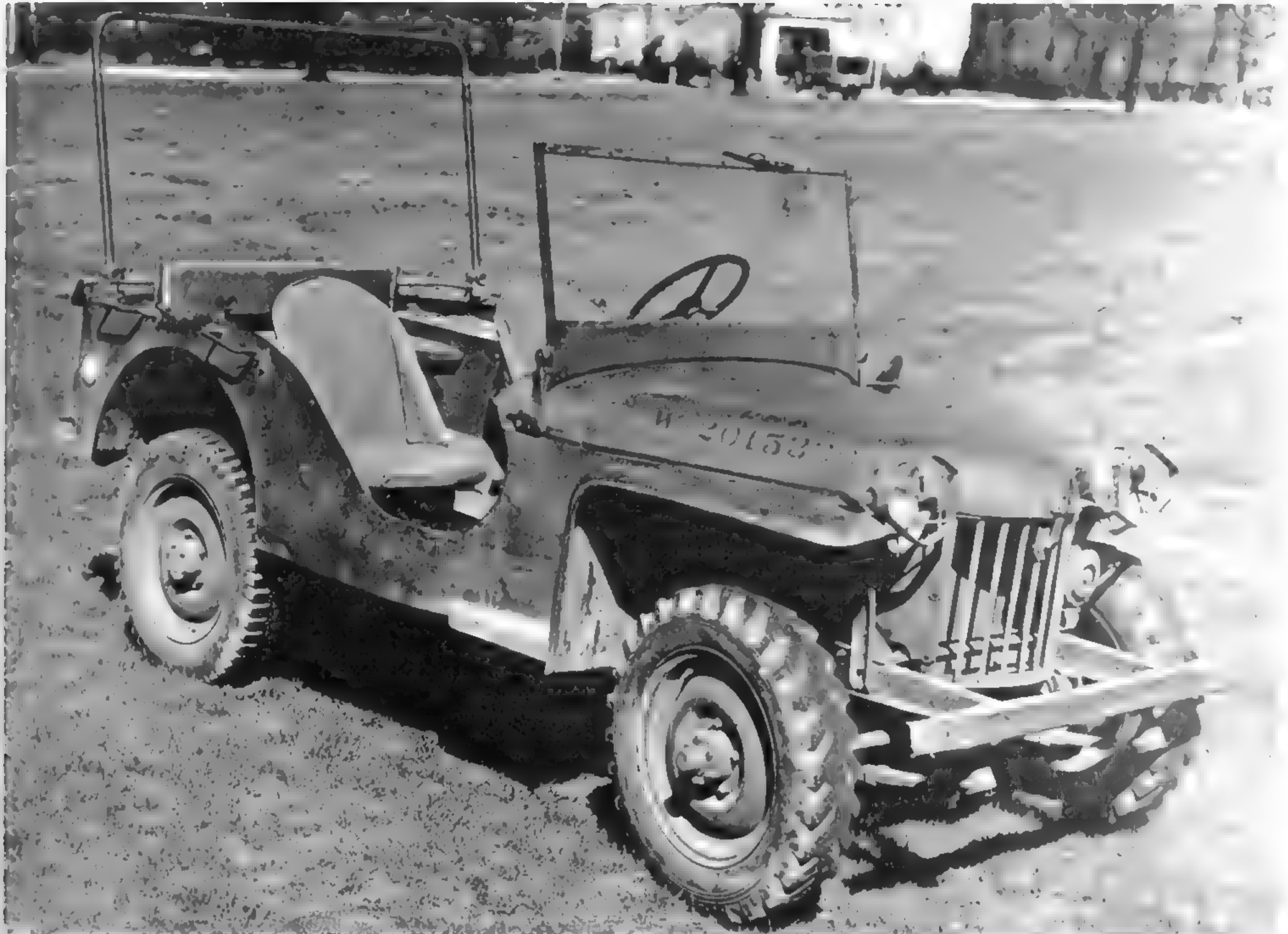
The Model 60 also included brush guards for the headlights. The windshield was replaced with a two-pane version on later models. (National Archives and Records Administration photo)
